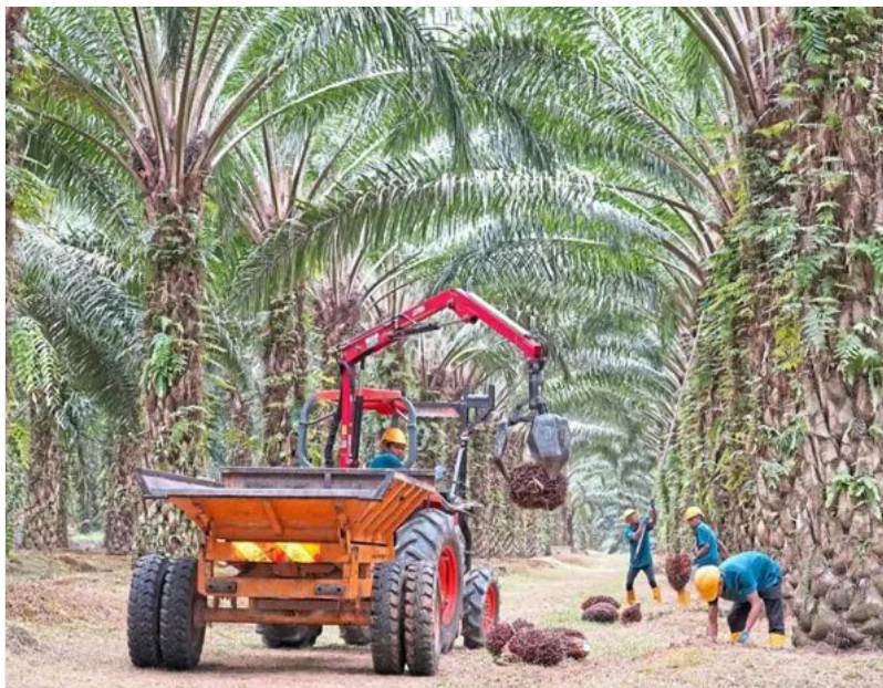
Boom harvester in action within oil-palm rows - enhancing safety and harvest efficiency in mature plantations. Photo by PalmINNOV
